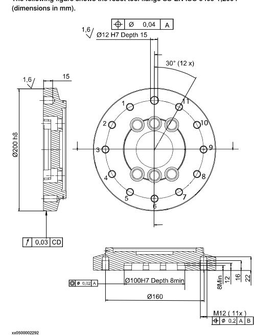
The following figure shows the robot tool flange SS-EN ISO 9409-1;2004
